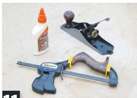
**11** Rear tote on this No.4 plane broke in half when removed. Clean up surfaces to be joined and re-glue
